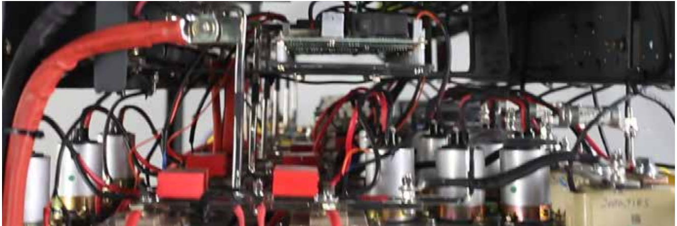
IGBT based, DSP controlled, low harmonics topology
