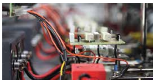
Smart Hybrid Power Module in Active Shunt topology
