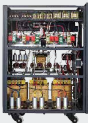
STATIC HIGH-SPEED VOLTAGE STABILISATION USING IGBT
